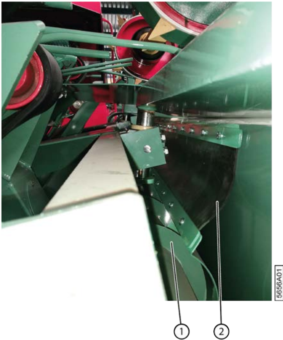
Fig. 144: Checking the condition of the rubber flap on the screw conveyor
