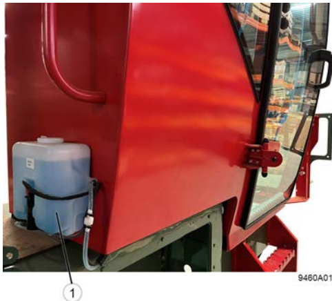
Fig. 114: The windscreen washer reservoir
