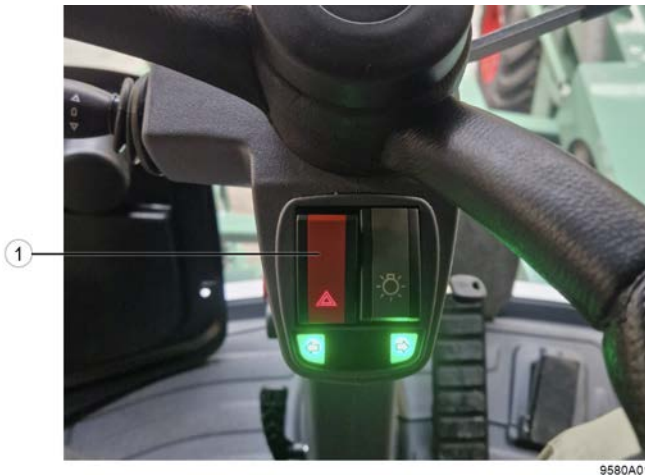
Fig. 71: Switching on the hazard lights
