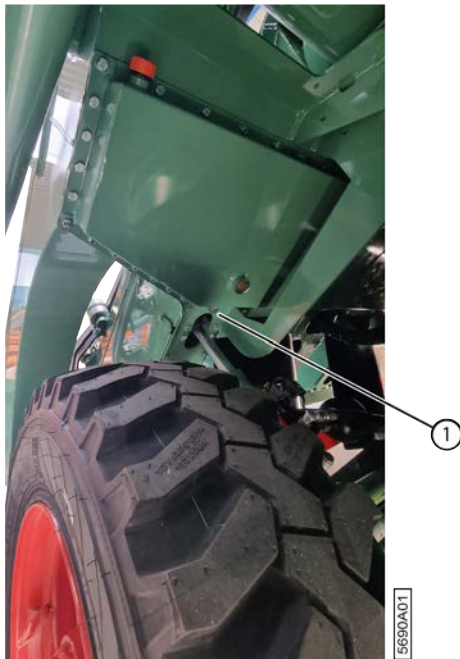
Fig. 143: Draining oil gearbox picking element
