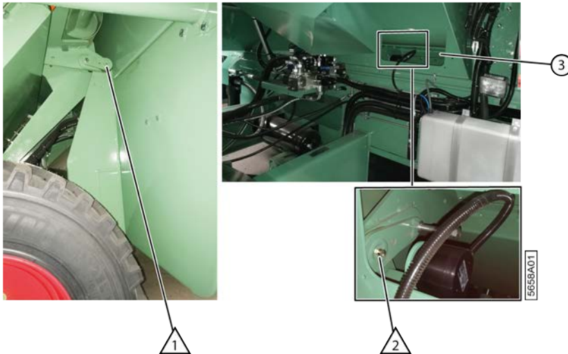
Fig. 146: Lubricating the pivot points of the picking element
