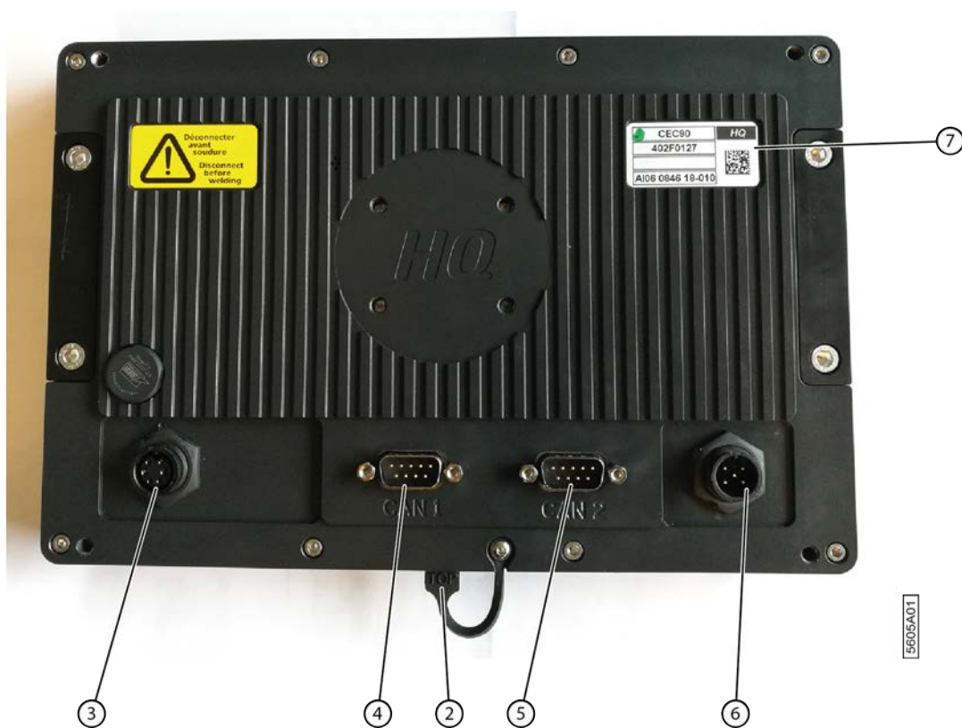
Fig. 69: The control screen (rear)
