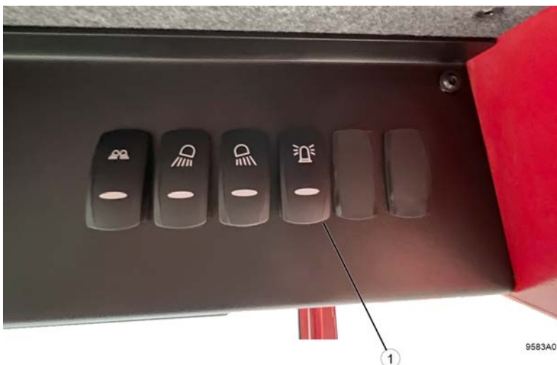
Fig. 72: Switching ON the beacon light
