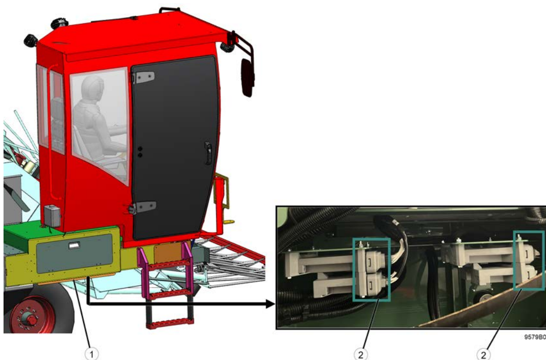
Fig. 160: The location of the controllers
