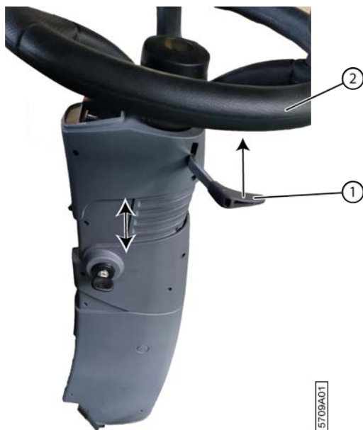
Fig. 87: Adjusting the height of the steering wheel
