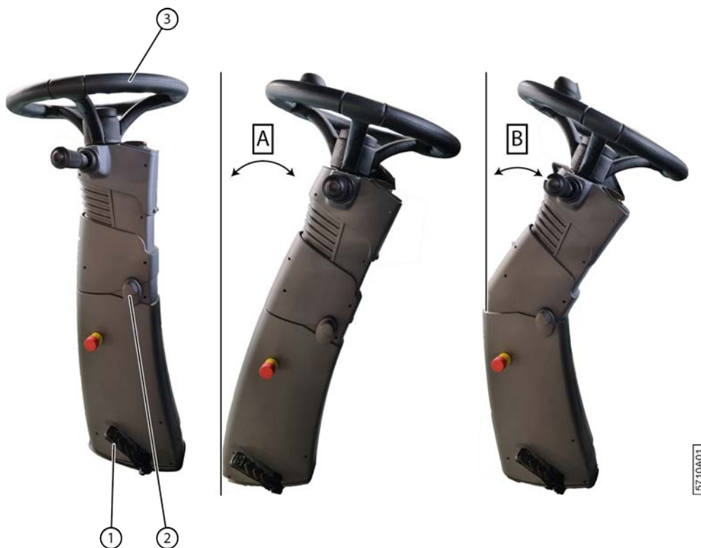
Fig. 88: Tilting the steering column
