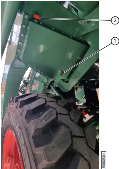
Fig. 142: Topping up the oil in the gearbox of the picking element
