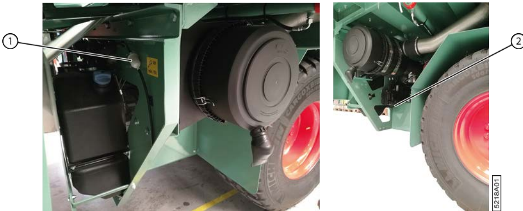
Fig. 174: Location of the AdBlue filters
