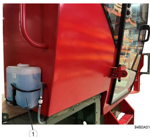
Fig. 18: The windscreen washer reservoir
