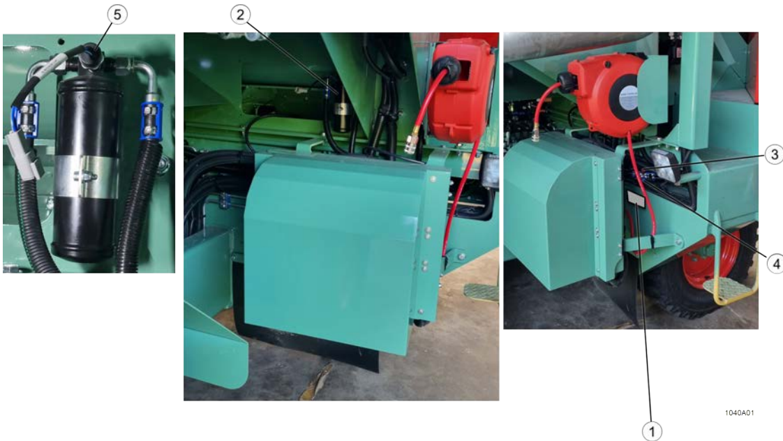
Fig. 116: The location of the air conditioning components
