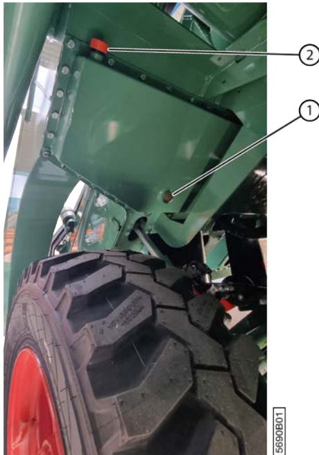
Fig. 141: Topping up the oil level in the gearbox for the picking element
