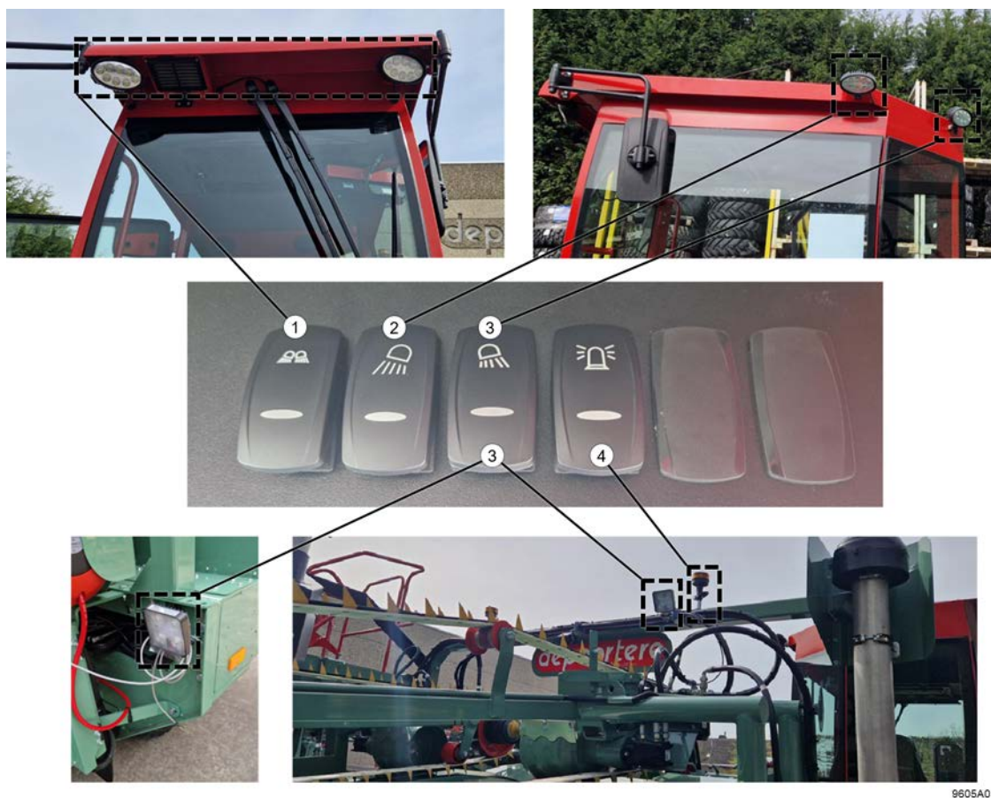
Fig. 70: The operating controls for the work lights and beacon light
