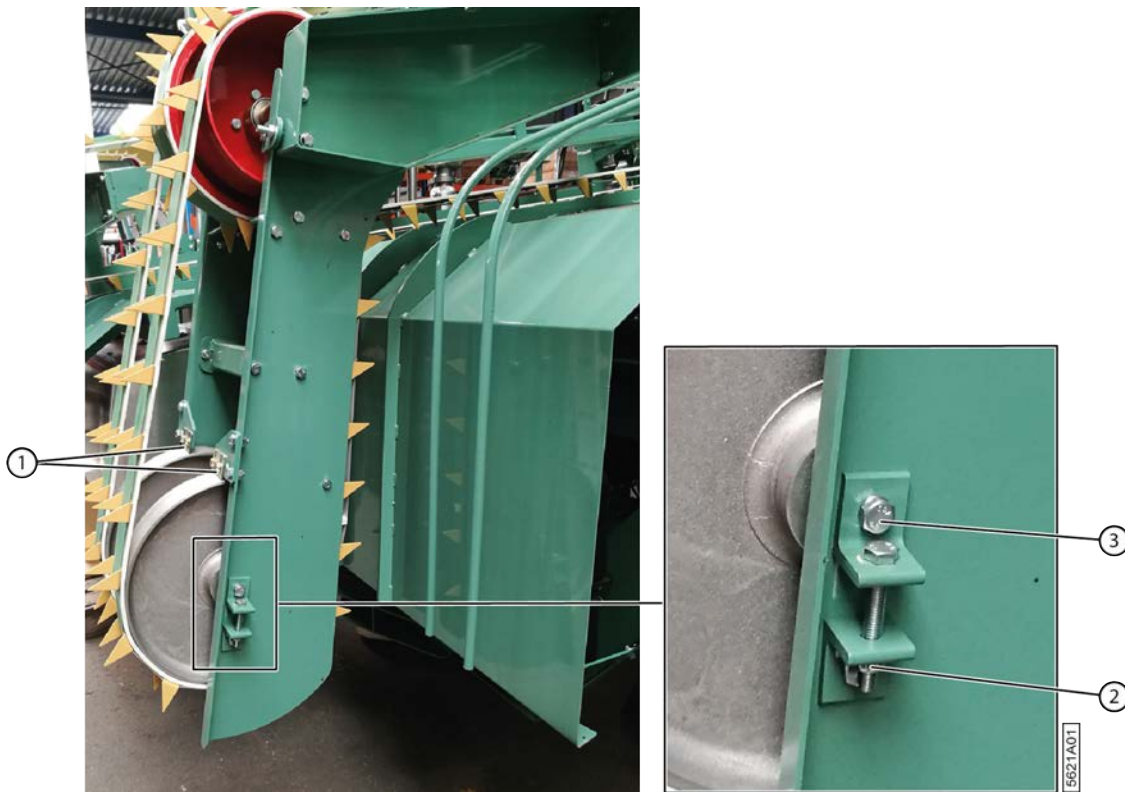
Fig. 98: Adjusting tension of the flax-laying belts
