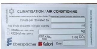
Fig. 117: The sticker with information about the air conditioning
