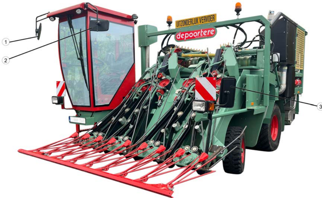
Fig. 15: The location of the mirrors
